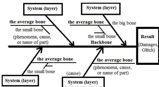
Fig 2: Diagram of identifying the cause of a complex problem
