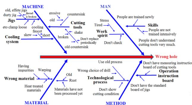
Fig 6: Determine the causes of hole defects
